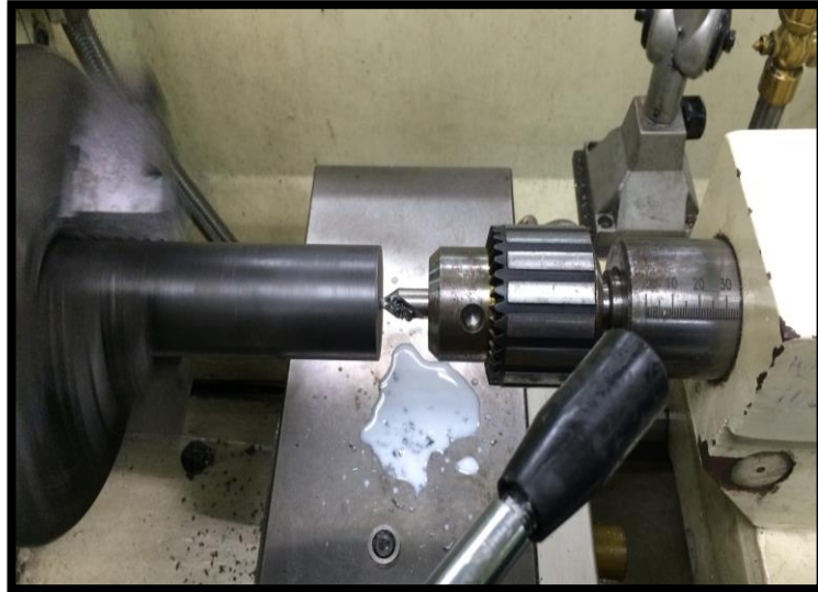
Figure 0.5: Centre drilling process
