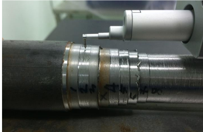
Figure 0.10: The uses of stylus at the contact surface of workpiece
