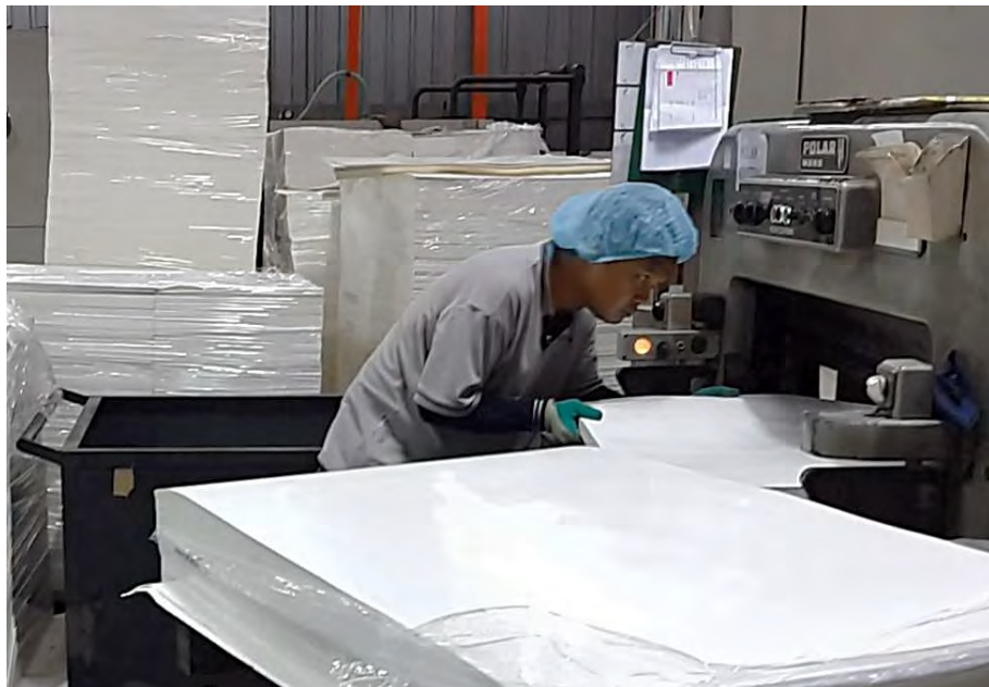
Figure 1.2: Polar cutting process performed by the operator using a polar cutter machine.
