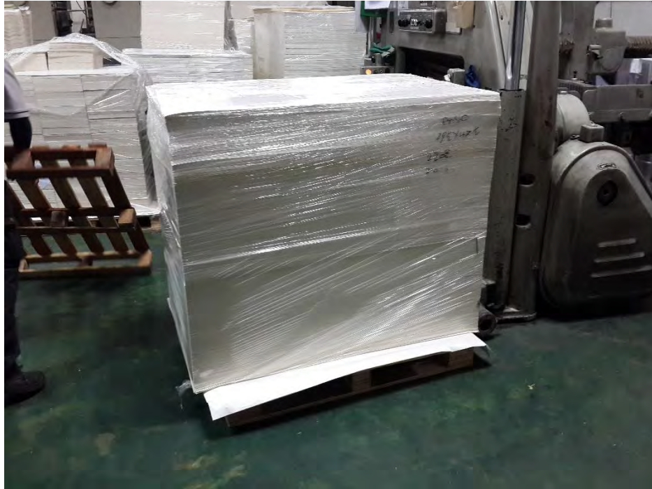
Figure 1.1: Paper stacks that used to make paper cups before polar cutting process.
