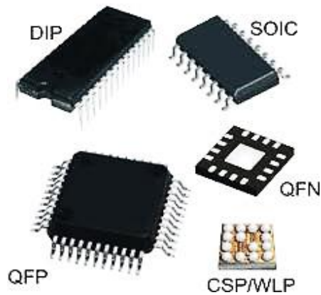
Figure 2.1: Type of IC Package (Diego & Development, 2001)
