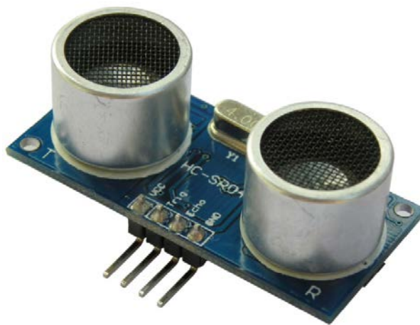
Figure 1.2: Ultrasonic sensor commonly used in mobile robot
