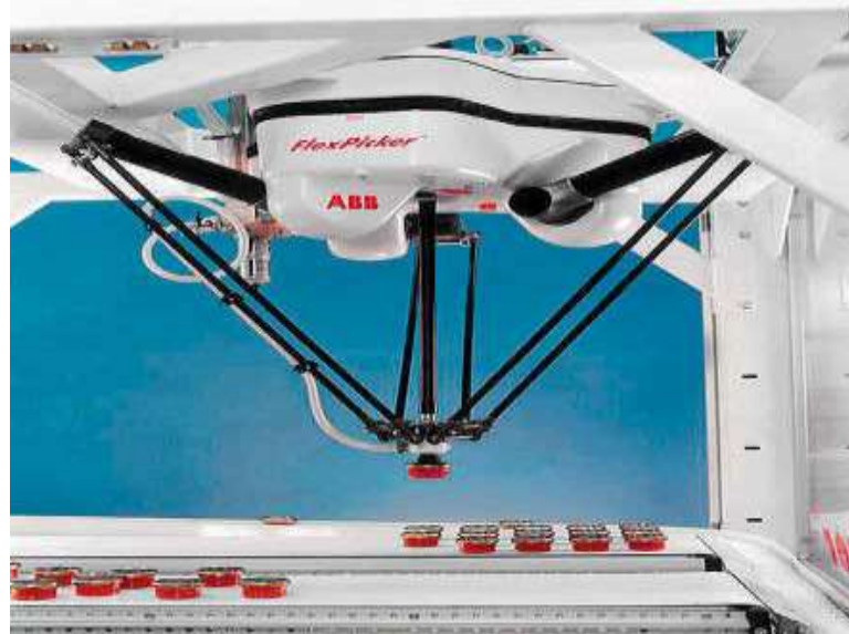
Figure 2.2: Pick and place operation of FlexPicker IRB 340 (Hanover, 2004)
