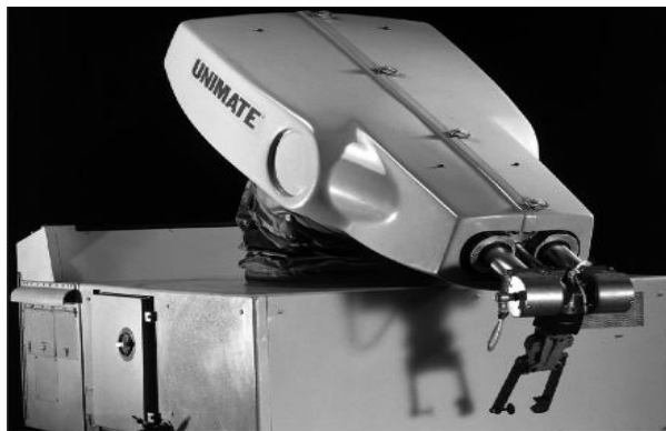
Figure 1.1: The first prototype of automotive robot built in 1959- the Unimate #001 (Royakkers, 2015)
