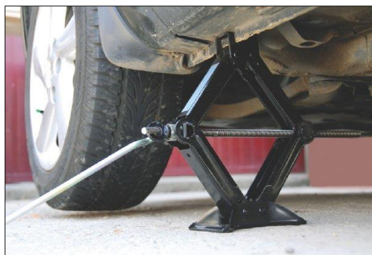
Figure 1.2: Notch underneath the car to fit the car jack
