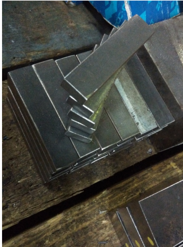
Figure 1.1: Steel plates after squaring process in manual milling operation (Source: Multi-Precision Industries Sdn. Bhd., 2015)
