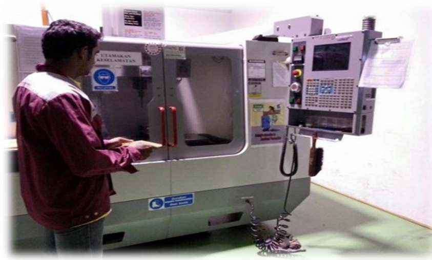
Figure 2.1: Process of Loading a work pieces for the HAAS VF-1 CNC Milling Machine
