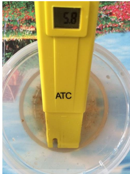
Figure 4.8: The pH Reading that Shows Appropriate Value for The Crop
