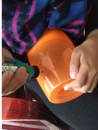
Figure 3.16: Process of Installing Float Switch in Vase
