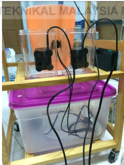
Figure 3.17: Process of Installing Water Pump in Tanks
