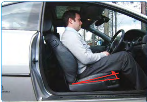
Figure 2.7: Adjust car seat pan angle to ensure driver's thighs can fully supported by the car cushion.
