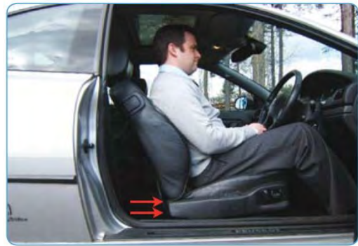
Figure 2.6: Move car seat forward until driver's feet can fully depress three pedals such as clutch, accelerator and decelerator.
