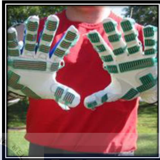
Figure 3.5: Eighteen sensors are attach to the glove (Source: www.tekscan.com )
