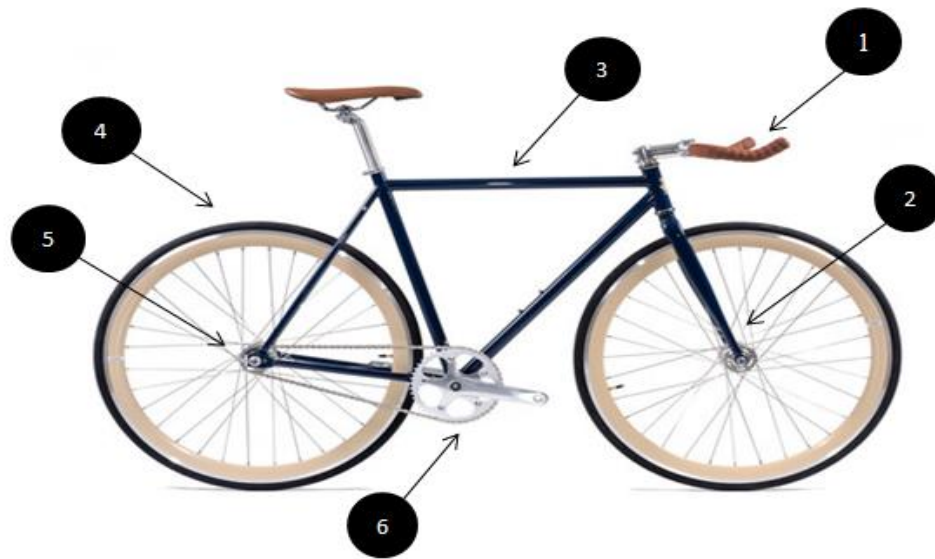
Figure 1.2: Fixed bicycle part; 1.Steering 2.fork 3.frame 4.wheel 5.rear sprocket 6.front sprocket (State Bicycle, 2016)
