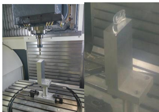
Figure 3.42: Roughing process with five axis machine
