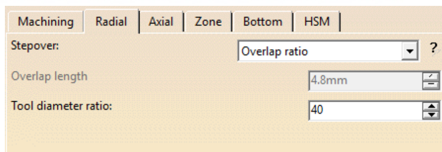
Figure 3.25: CAM setting of roughing operation 3, radial (Geometry Page)
