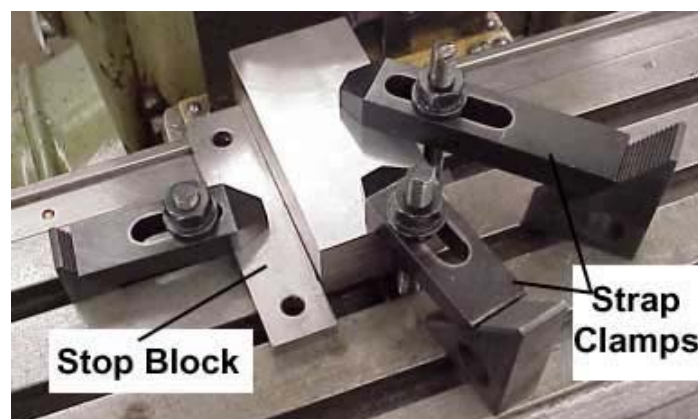
Figure 2.19 workpiece is clamp directly to the table[ retrived from http://archive.li/ru1r8/13b11e7835d22f2e9cf81d28a965f183439a1181.jpg ]
