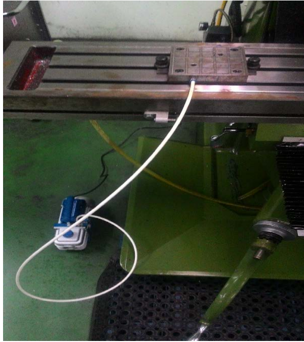
Figure 4.8 Vacuum clamping connected to vacuum pump
