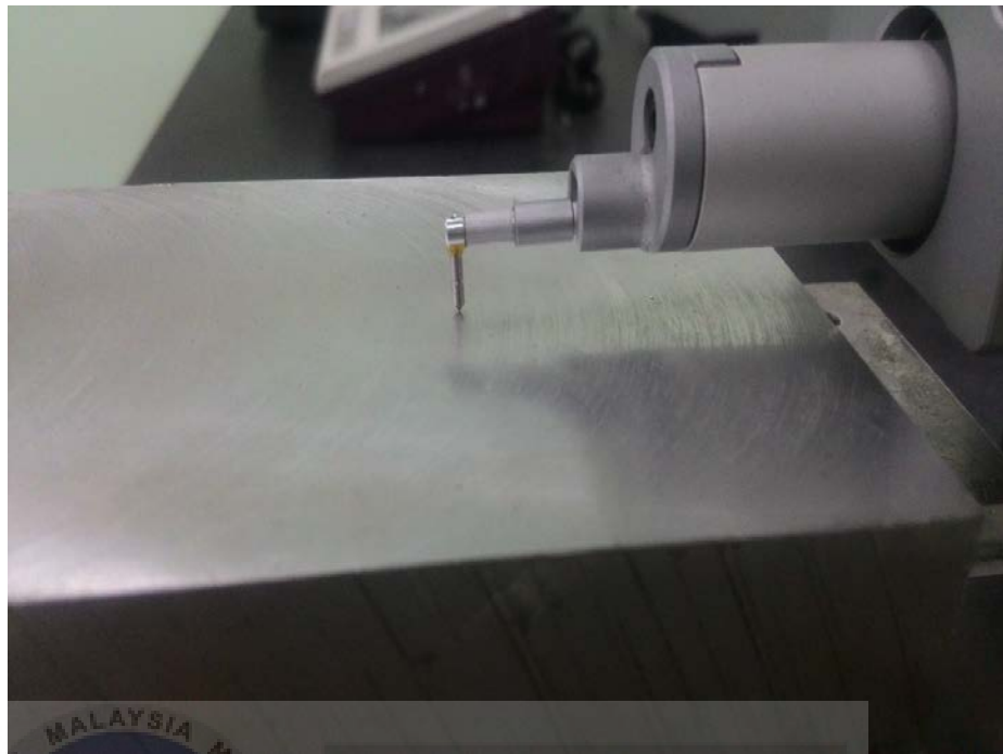
Figure 4.16 Surface roughness testing on aluminium workpiece
