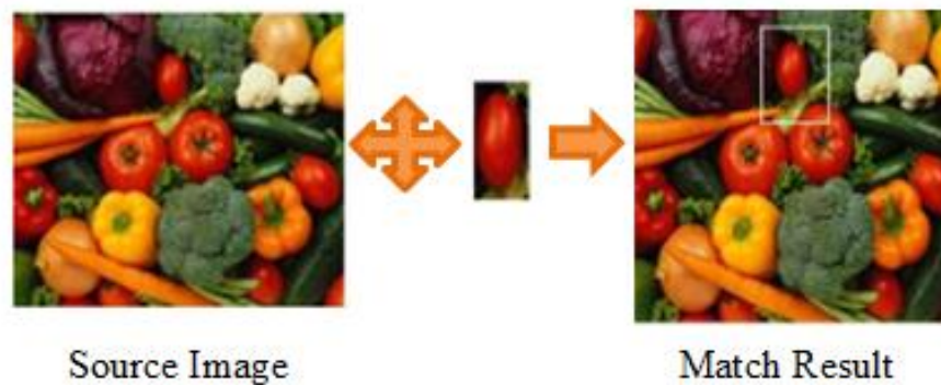
Figure 2. 7 :Process of template matching (Kumar et al., 2014)
