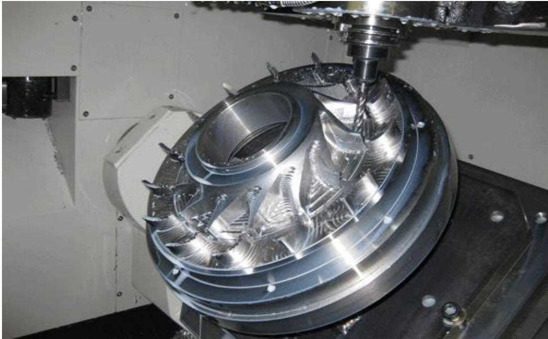
Figure 1.0: Five-axis machining performed for complicated part.
