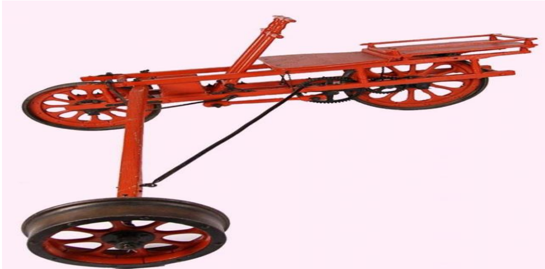
Figure 2.3: The 3-wheeled Velocipede Hand Car
