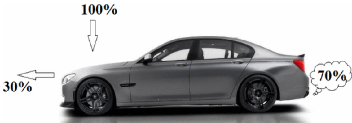
Figure 1.2 Energy loss of a car
