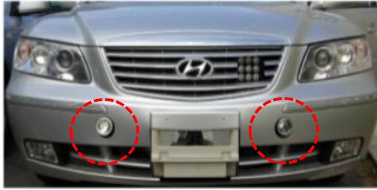
Figure 2.5: The laser scanner integration and the headlights.
