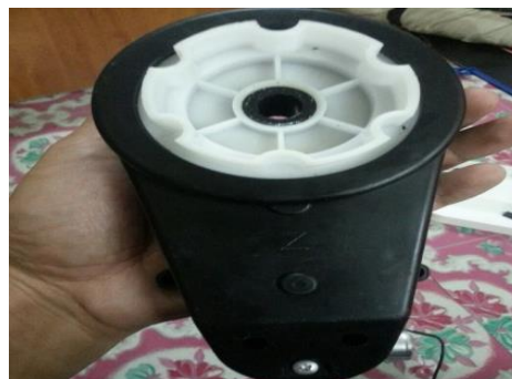
Figure 3.4 : Motor Gear box
