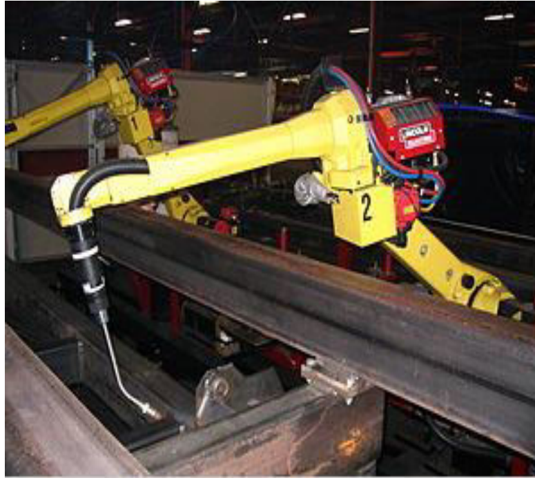
Figure 2.2: Example of Six-Axis Articulated Welding Robot Reaching into a Fixture to Weld [11]
