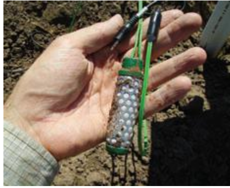
Figure 2.3: Moisture Sensor Type Resistance
