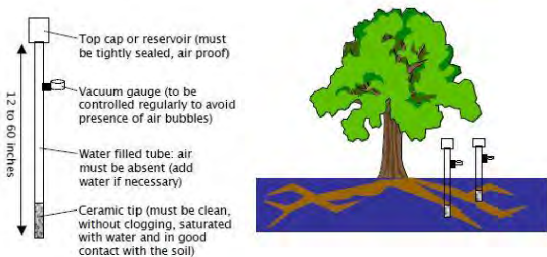
Figure 2.4: Diagram Of A Tensionmeter And A Station Of Two Tensiometers Installed At Different Soil Depths.
