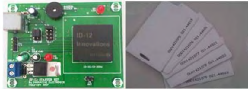
Figure 2.2.1: RFID Reader and Tags (D. Eridani & E. Widiyanto, 2015)
