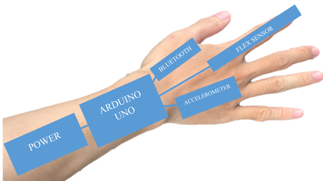
Figure 4.47: Simple Planning Design for Hand Gesture Glove Controller.
