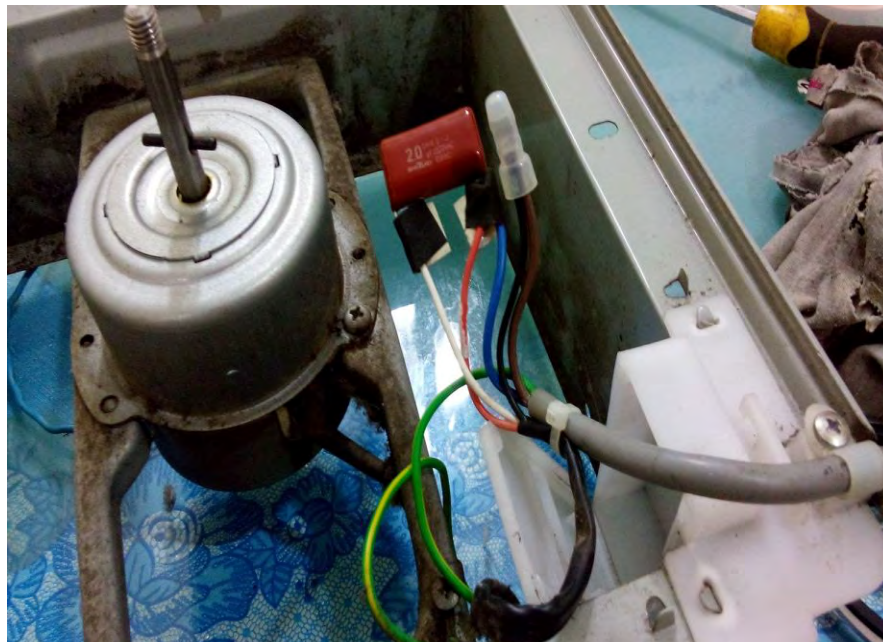
Figure 1.5: Single phase AC motor for exhaust fan Panasonic FV-20AUM8 (black wire - common terminal, white wire - start terminal, red wire - run terminal)
