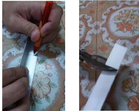
Figure 3.21: Marking and Cutting Aluminium Bar
