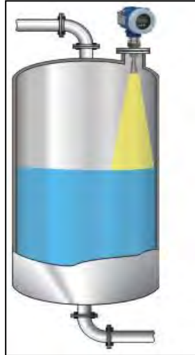
Figure 2.1 : Radar Level Transmitters(Anon n.d.)
