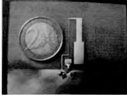
Figure 2.5: Antenna model for 868MHz
