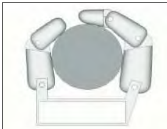
Figure 2.4: Model of second prototype grasping a cylinder with 2-segment of thumb [3]
