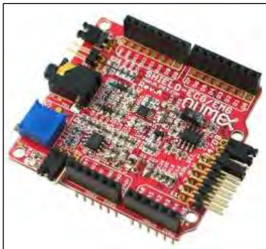
Figure 4.18: Olimex EKG/EMG shield.
