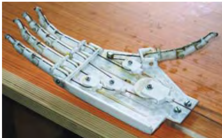
Figure 2.6: Mechanical hand design with one actuator [5].
