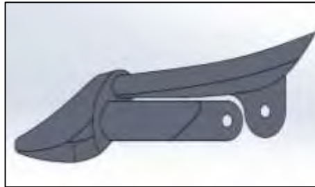
Figure 4.6: The prototype of finger design.
