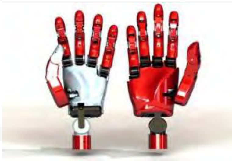
Figure 2.5: Image of multifunctional prosthesis hand [4]
