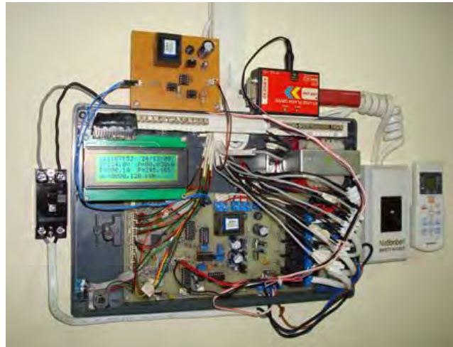
Figure 2.2: Main Controller box (Sittisak Rojchaya and Mongkol Konghirun, 2009)
