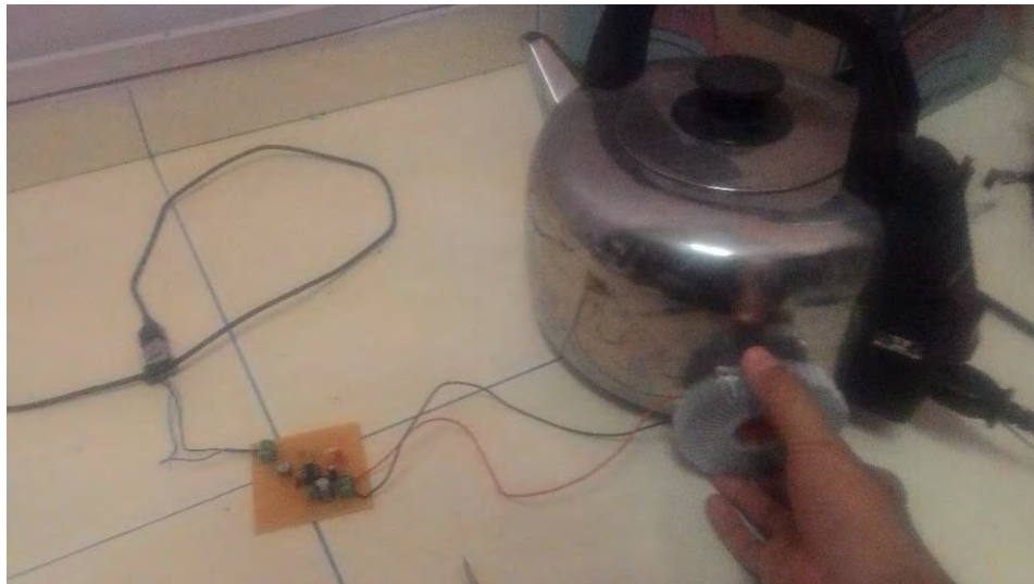
Figure 4.14: Circuit does not turn on when TEG is given heat from electric kettle.
