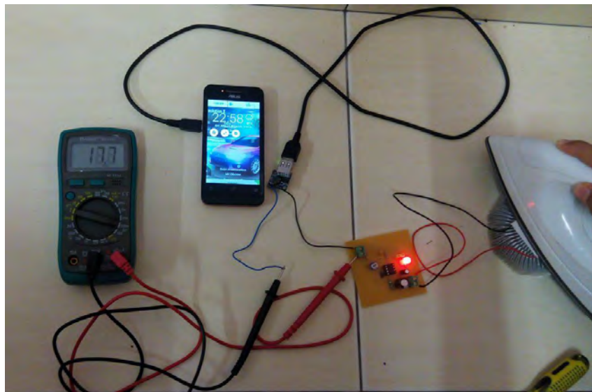
Figure 4.9: Measuring output current when charging phone.
