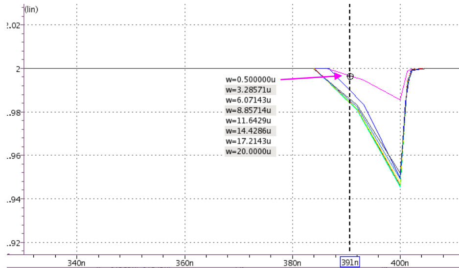
Figure 4.33: Parametric analysis for comparator circuit width seep from 0.15\mu\text{m} to 20\mu\text{m}
