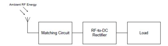
Figure 1.1: Block diagram of RF energy harvesting system
