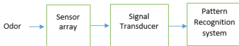
Figure 2.2: Working principle of E-Nose
