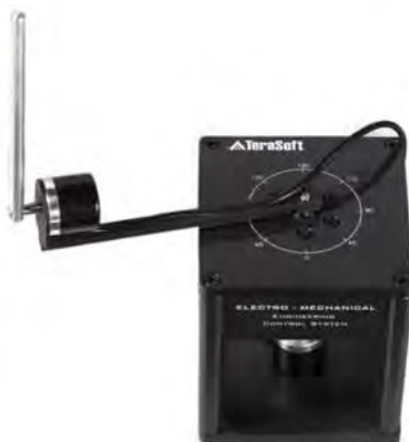
Figure 2.1: TERASOFT Rotary Inverted Pendulum
