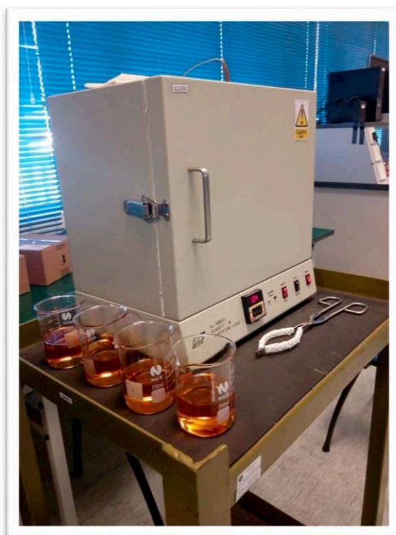
Figure 3.4.1 : Microwave used to heat the oil samples
