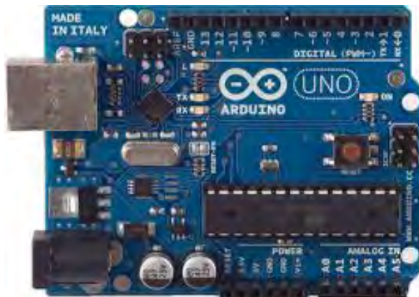
Figure 3.4: Arduino UNO board
