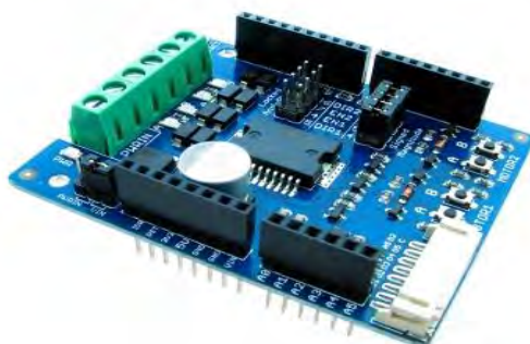
Figure 3.7: 2Amp Motor Driver Shield [15].
