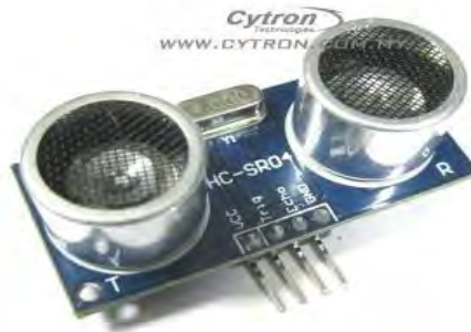
Figure 3.2: Ultrasonic Sensor HC-SR04 [9].
