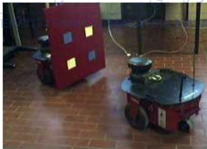
Figure 2.1: Pioneer 2DX Mobile Robots [3]
