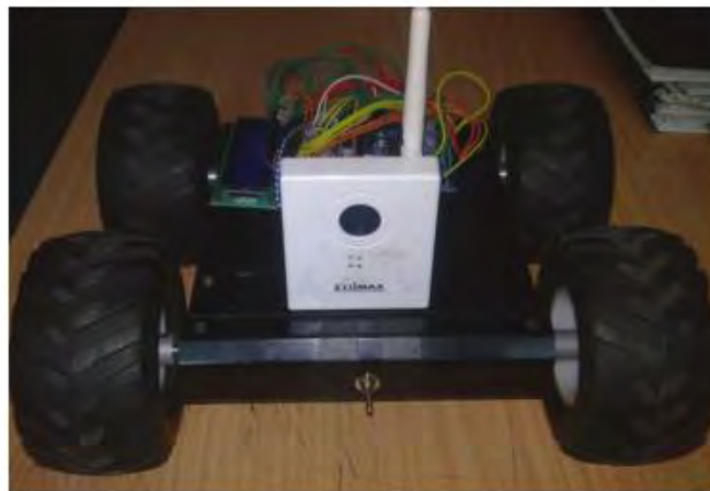
Figure 2.5: Mono- camera used on a mobile robot[10].
