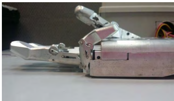
Figure 3.28: Pinky finger of the bionic hand bends
