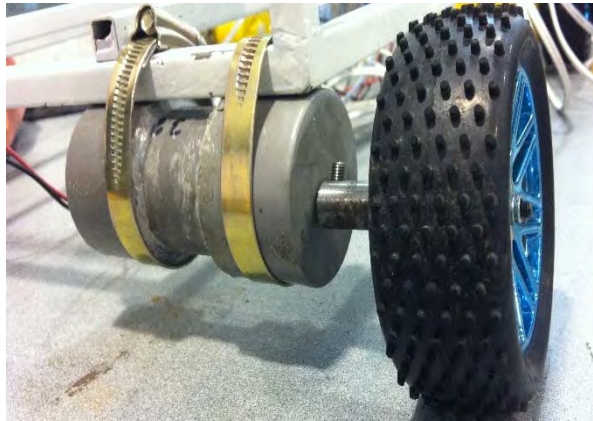
Figure 3.9: DC geared motor with wheel of tire
