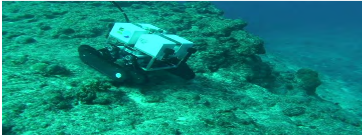
Figure 2.2: Small size flipper type crawler ROV running on the steep rock reef [1]
