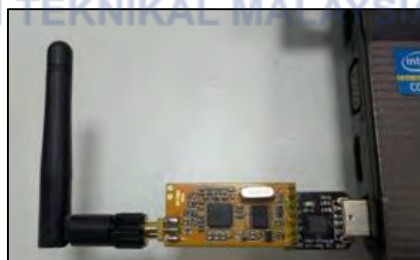
Figure 3.23: The attachment of APC220 module into PC/laptop
