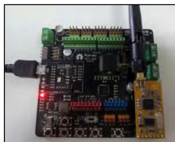
Figure 3.24: The attachment of APC220 module into Arduino board
