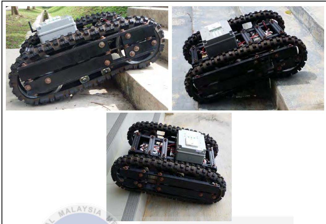
Figure 4.24: Obstacle test on difference heights of ladder
