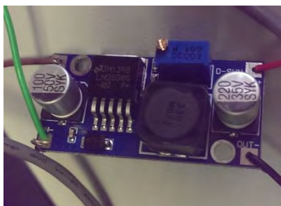
Figure 3.25: Step down voltage regulator
