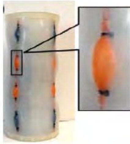
Figure 2.17: Active modular elastomer for soft wearable assistance robots designed by Park et al. (source: Recent Trends in Lower-Limb Robotic Rehabilitation Orthosis: Control Scheme and Strategy for Pneumatic Muscle Actuated Gait Trainers) [21]
