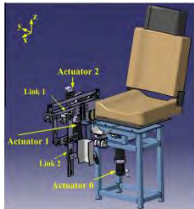
Figure 2.12: Lower limb rehabilitation system designed by Erhan Akdogan [18]
