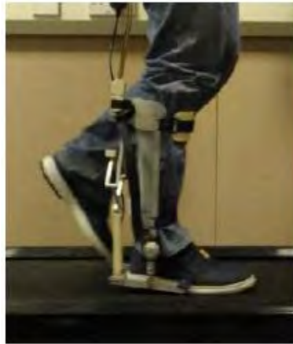
Figure 2.15: Active ankle-foot orthosis (AAFO) designed by Carberry et al. (source: Recent Trends in Lower-Limb Robotic Rehabilitation Orthosis: Control Scheme and Strategy for Pneumatic Muscle Actuated Gait Trainers) [21]
