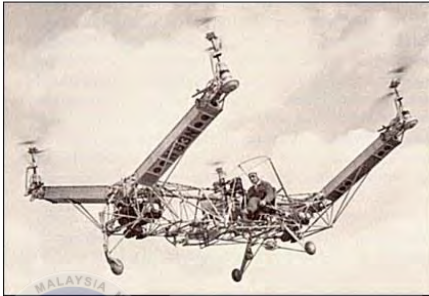
Figure 1.1: Convertawings Model A. First Quadrotor that able to fly [2]
