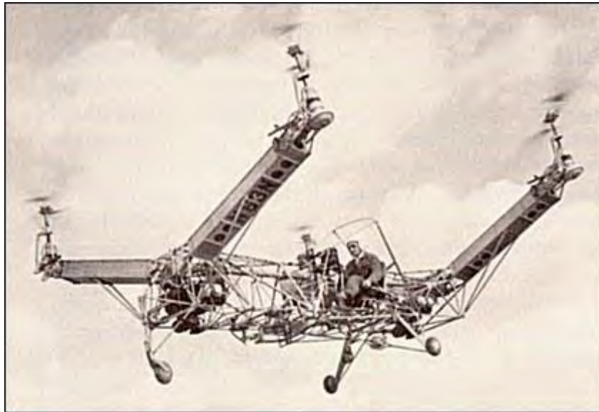
Figure 1.1: Convertawings Model A. First Quadrotor that able to fly [2]
