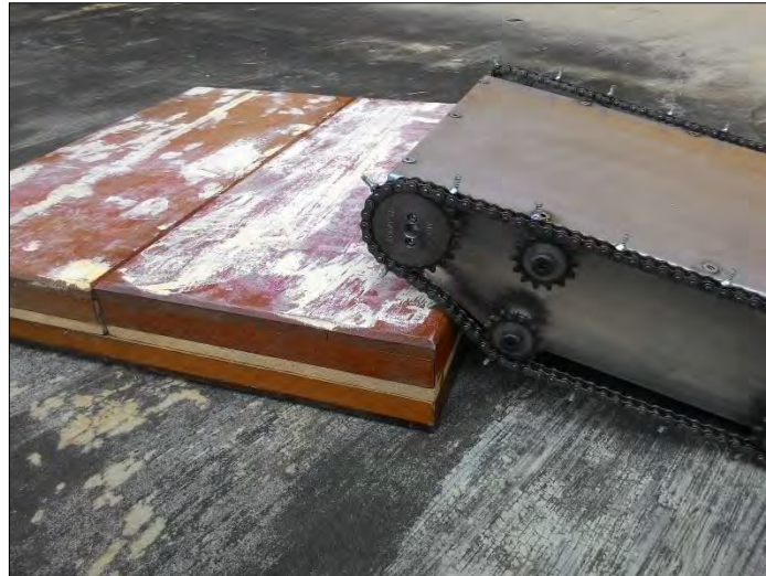
Figure 4.12: The crawler climbed the 9.5 cm obstacles.
